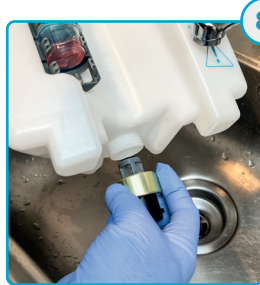
Skrue filteret af Unscrew the filter
