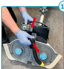
Tag sugeslangen af Remove the suction hose
